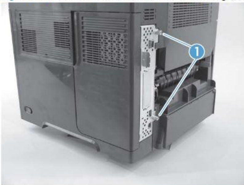
Figure 2-13 Remove the formatter cover and formatter cage (2 of 3)
