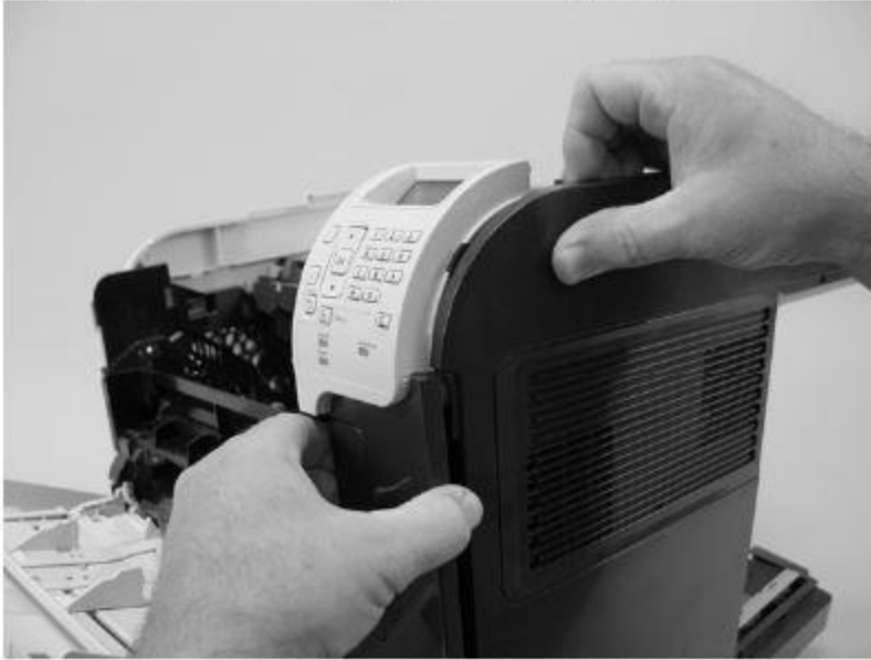
Figure 2-46 Remove the right-side cover (2 of 3)
