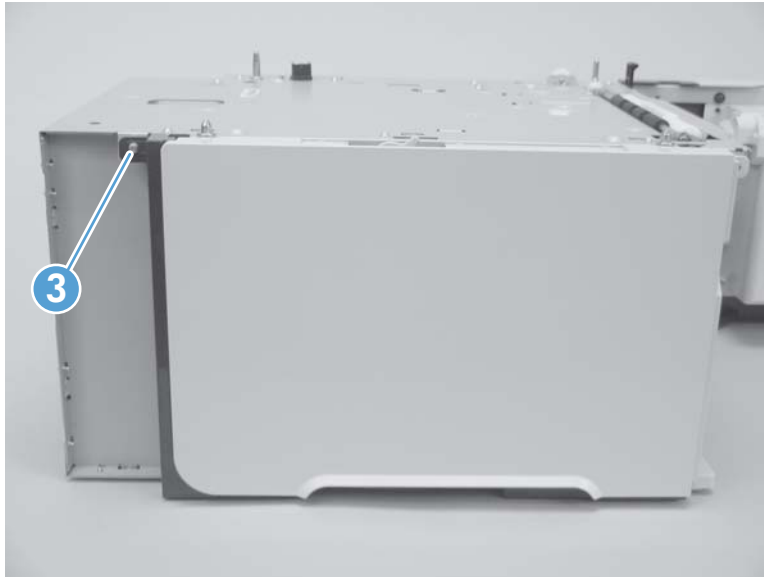
Figure 2-146 Remove the left-side cover (PD; 4 of 5)
