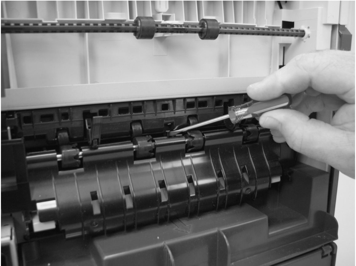
Figure 3-6 Test the fuser delivery sensor (PS700)
