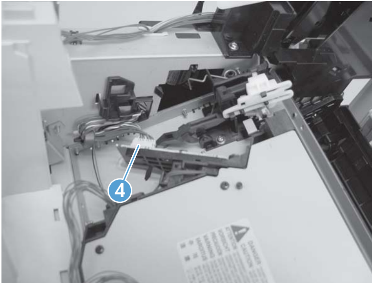
Figure 2-131 Remove the laser/scanner assembly (4 of 4)
