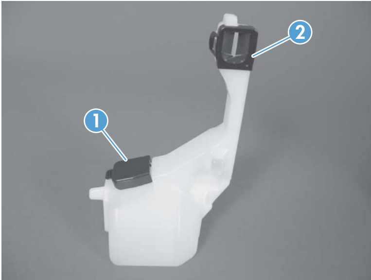
Figure 1-14 Remove the toner-collection unit (4 of 4)
