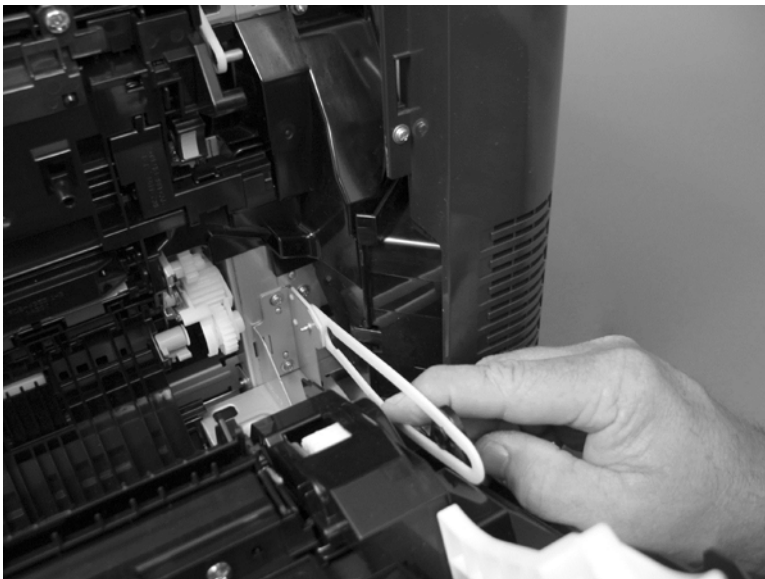
Figure 1-76 Remove the right-door assembly (4 of 8)
