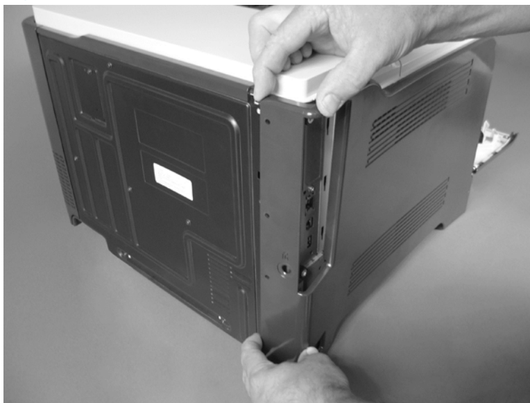
Figure 1-85 Remove the left cover (2 of 5)
