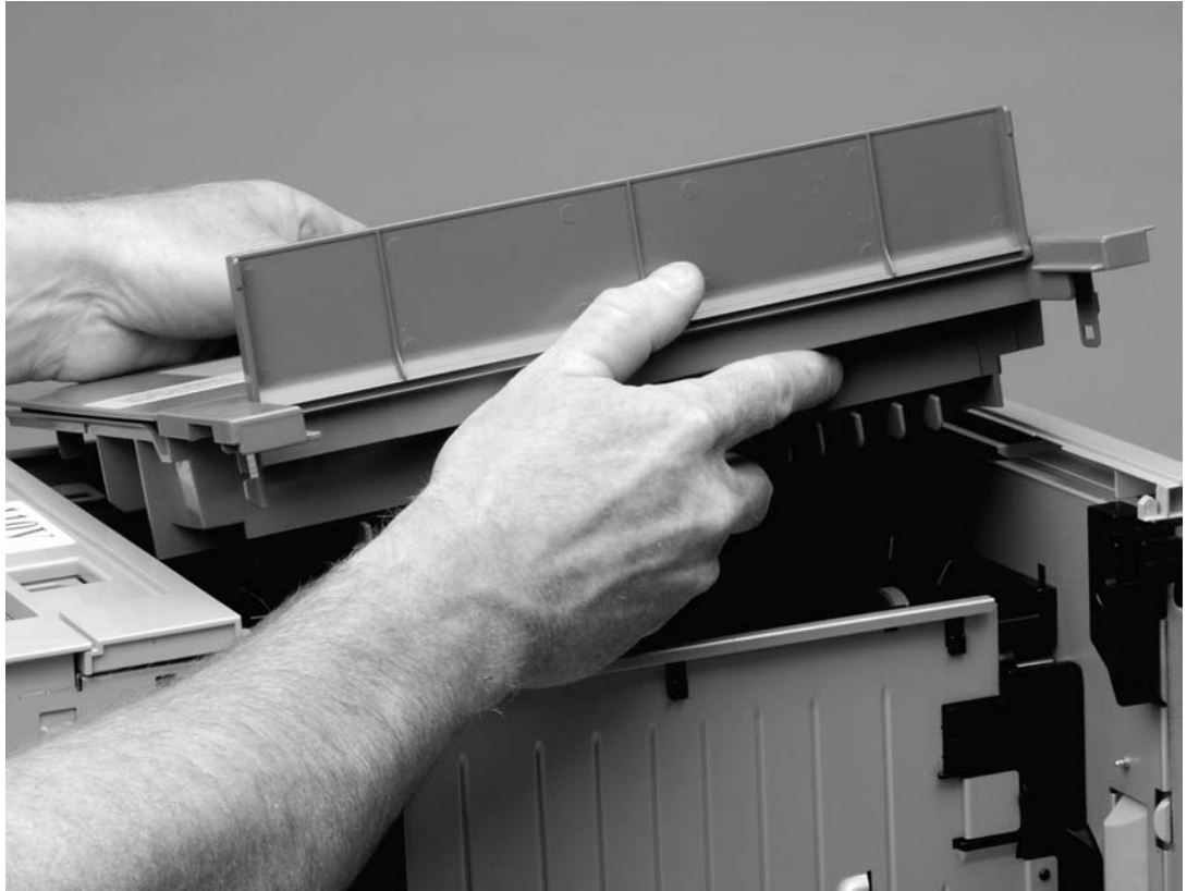
Figure 6-5 Removing the back cover (3 of 3)
